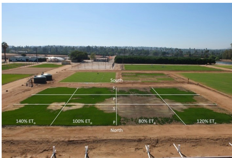
Figure 1. Bermudagrass salinity alleviation research area showing suction lysimeters on turf surface prior to insertion below the turf surface. Two 5,000-gal tanks are used to store and deliver saline irrigation water. Riverside, CA.
