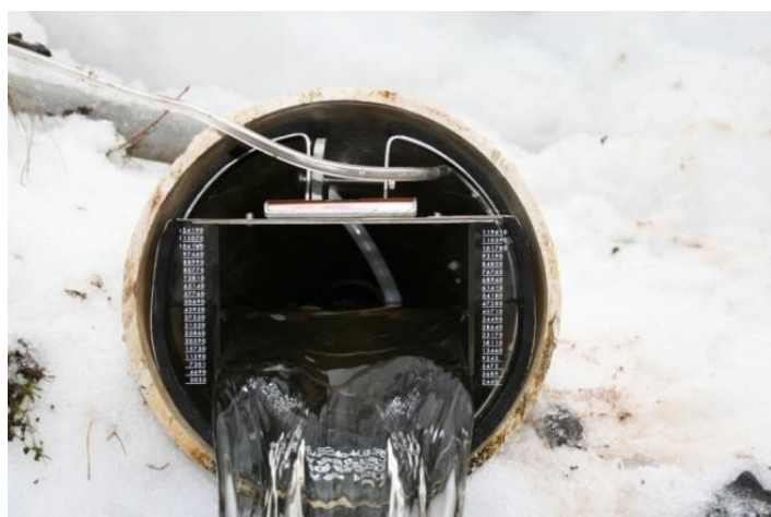
Figure 3. Compound weirs in the outlet of the west (control) and east (treatment) drainage lines at Northland Country Club.
