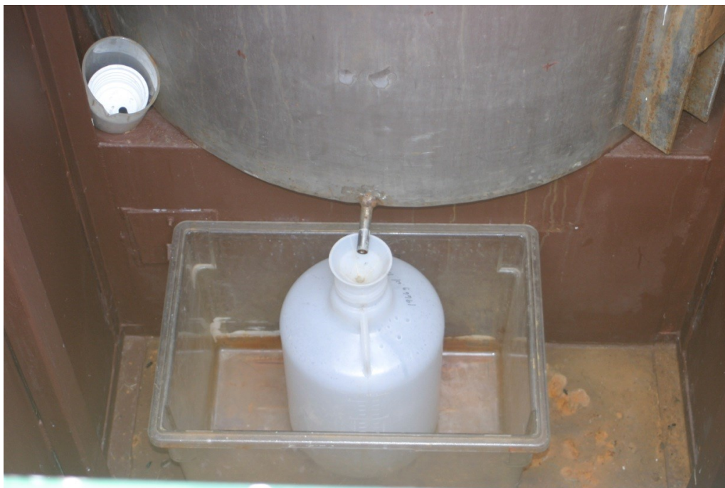
Figure 2. Water leachate is collected on a regular basis to measure the amount of nitrogen and phosphorous that leaches through a Kentucky bluegrass turf maintained at rough height.
