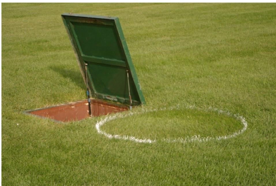
Figure 1. The white circle in the foreground marks the top of a large lysimeter used to measure the amount of nitrogen and phosphorus that leaches through a 22-year old turf. The raised hatch allows researchers to collect samples at the base of the lysimeter.
