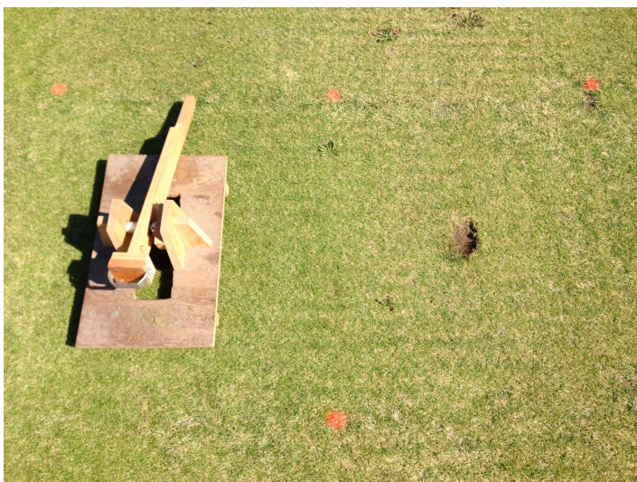
Figure 2. A divot-cutting device was used to remove divots from both trafficked and non-trafficked plots. (photo credit: Maggie Reiter)
