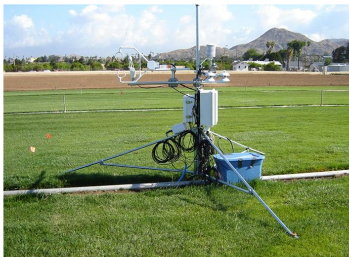
Figure 5: Whole field eddy covariance systems for measuring water and CO 2 , installed above turfgrass. Three turfgrass sites were established in 2013.
