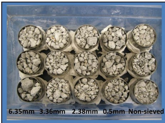
Figure 2. Picture of the various sized fractions of slag samples tested for hydraulic conductivity. Size fractions included >6.35, >3.36, >2.38, >0.5 mm, and non-sieved.
