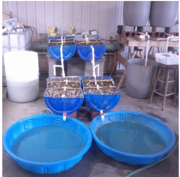
Figure 1: Laboratory S2BR bioreactors could provide a natural, low cost method to treat waste water and provide.
