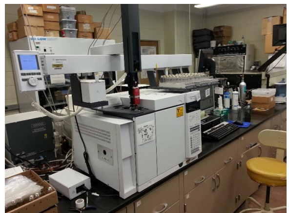
Figure 2. Gas chromatograph used to sample the greenhouse gases.
