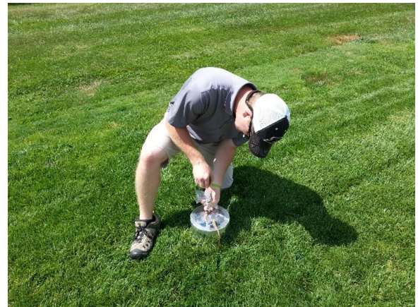
Figure 1. Sampling from the greenhouse gas flux chambers.
