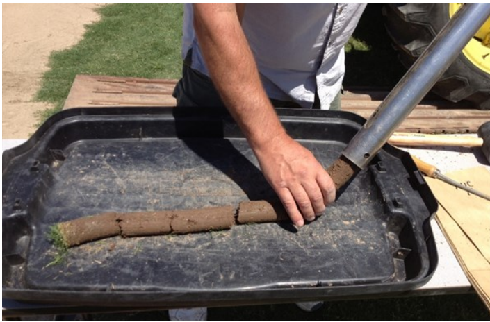
Figure 2. Soil samples being removed from sample tube. Samples were divided into 1' increments then analyzed for cation exchange capacity, exchangeable sodium percentage and soil salinity.
