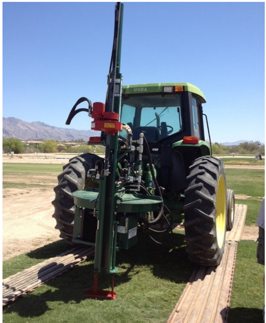
Figure 1. Soils were sampled to a depth of 3' in April using a Giddings Probe.
